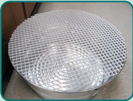
Figure 5. Grate cut to fit basin.
