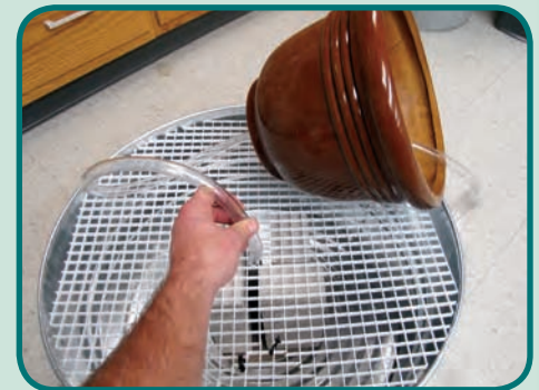
Figure 10. Cut a hole in the grate and mesh for the flexible tubing.
