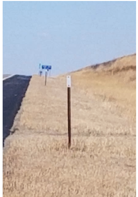
Figure 3. Total vegetation control around delineator posts facilitates mowing. Photo credit: Frannie Miller
