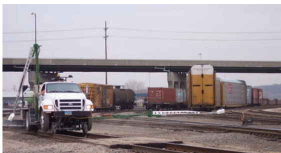
Figure 8. Trucks with the ability to move on roads or rail are commonly used to treat railroad ballasts. Photo credit: Nic Zimprich
