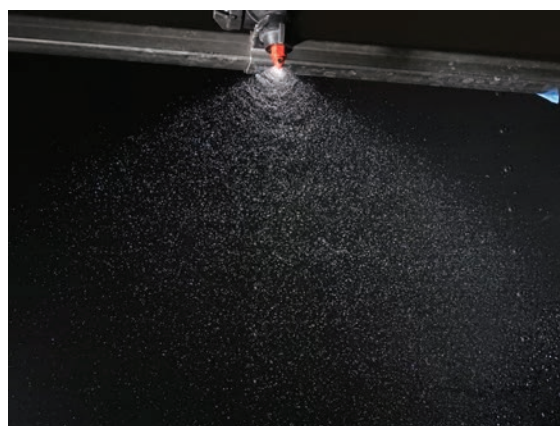
Figures 1-3. These images show the difference in droplet size based on the type of nozzle selected. Nozzle: AI XR 11004 (air inclusion 110-degree flat fan coarse spray); XR 11004 (flat fan medium/fine spray); and TTI04 (Turbo Teejet Extra coarse spray). Photo: Mark Ledebuhr, Application Insights, LLC 2020, www.bugwood.org
