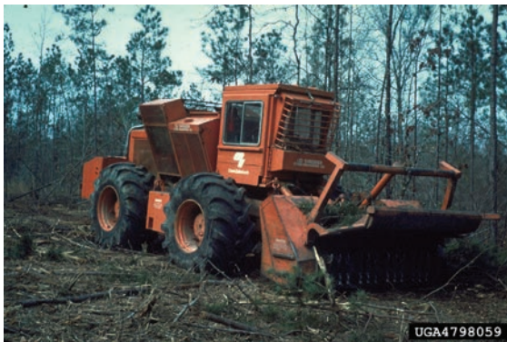
Figure 4. Mechanized equipment used to remove large trees on the right-of-way. Photo: David M. Moehring, Mississippi State University, www.bugwood.org
