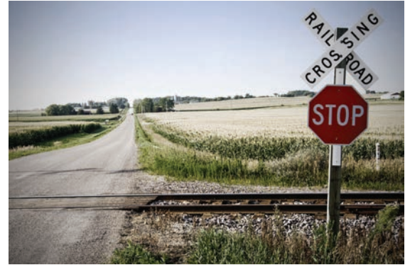
Figure 13. At railroad crossings, both the train and the traffic must be visible.
