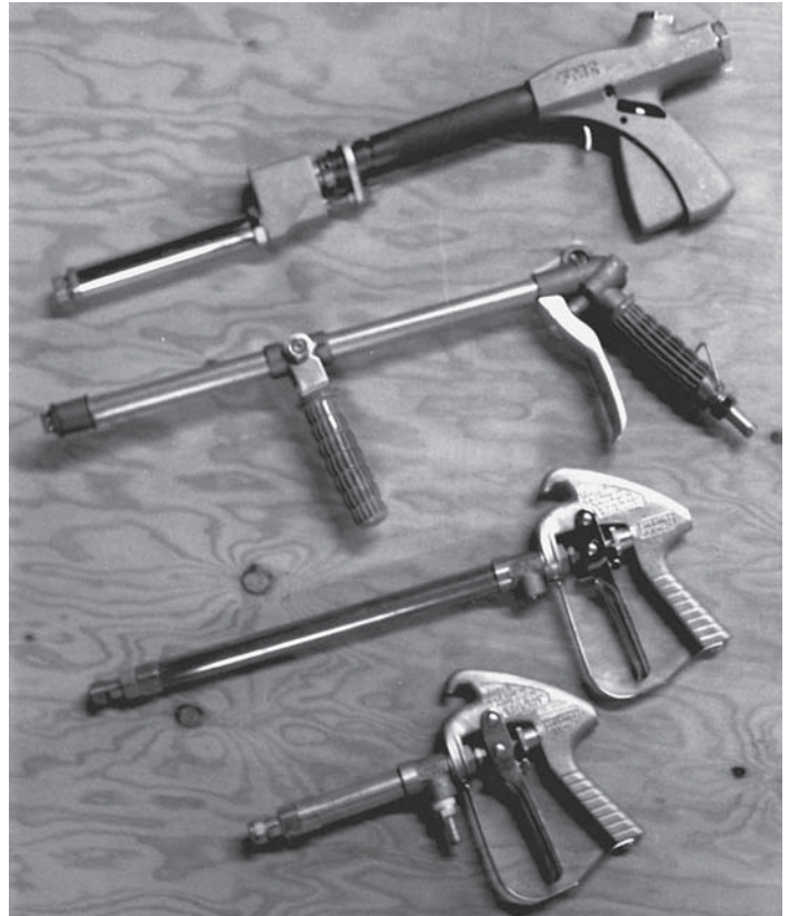
Figure 3. The flow capacity of agricultural spray nozzles varies greatly. Of those pictured, only the top (FMC #785) and the second (FMC #240 of Hypro #3381-0010) are rated above the 6 gpm at 125 psi.
