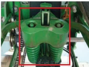
Figure 1. Mechanical spring (within red box) for downforce control.
