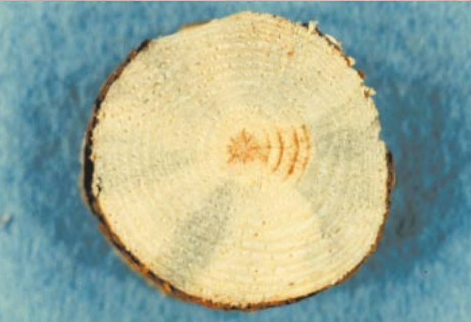
FIGURE 7 Sectors of cobalt-blue discoloration in a Scots pine log, caused by blue-stain fungi.
