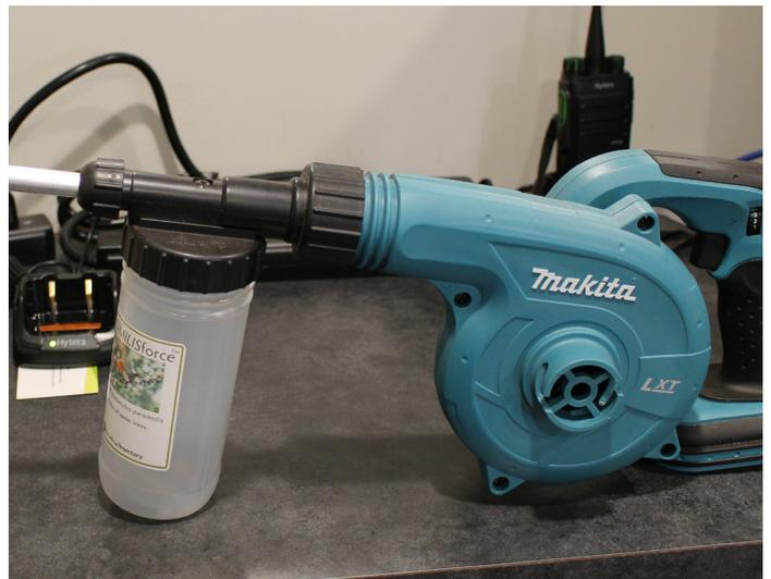
Figure 10. Mechanical blower used to apply *Phytoseiulus persimilis* throughout the greenhouse (Raymond Cloyd).
