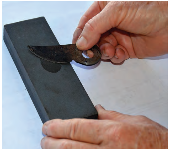
Figure 4: Lubricate constantly to prevent the pores in the whetstone from becoming clogged with metal shavings and to reduce heat from friction while sharpening.
