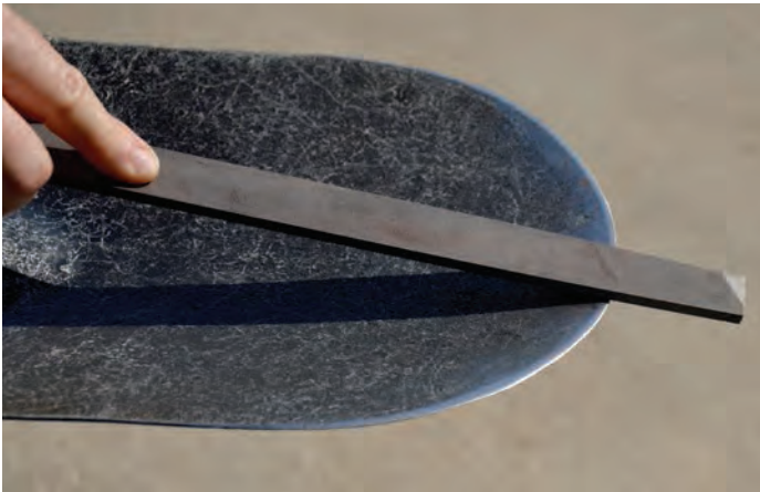
Figure 5: Bevel the front edge using a hand file or grinder.
