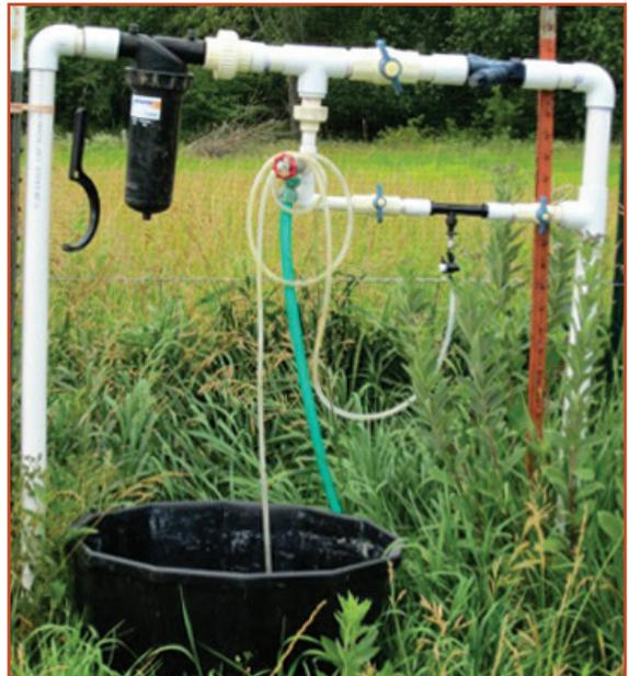
*Figure 2.* A venturi-type injector introduces fertilizer into the irrigation water.
