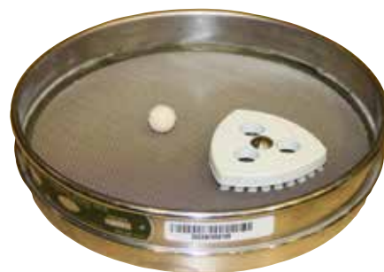
Figure 3. Example of one rubber ball and one bristle sieve cleaner.
