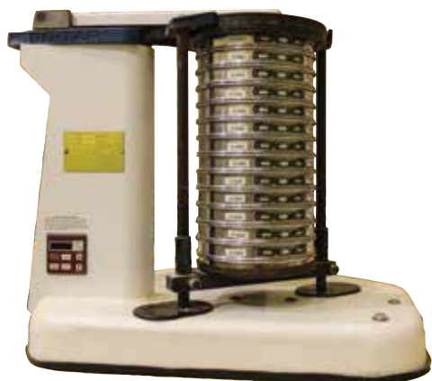
Figure 2. Tyler Ro-tap shaker machine with sieve stack.
