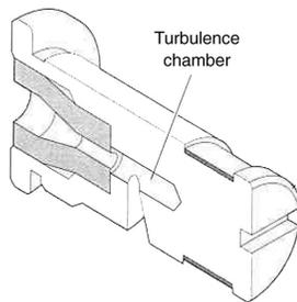
*Pre-orifice flood nozzle with turbulence chamber*
