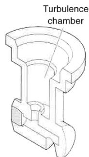
*Pre-orifice turbo flat-fan nozzle*
