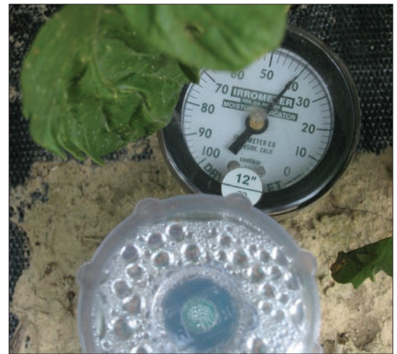
Figure 11. A tensiometer can be used to monitor soil moisture.
