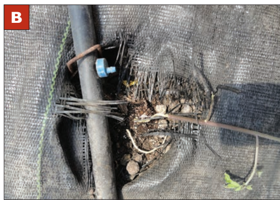
Figure 4. In high-pressure drip systems, emitters are either (A) preinstalled at the factory or (B) installed during assembly.
