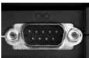
Figure 1: Nine-pin RS-232 connector.
