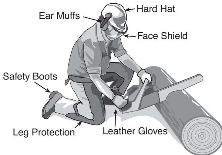
Select a chain saw with good safety features, including features to reduce kickback and an anti-vibration system to reduce saw vibration to the user's hands. This reduces user fatigue and ensures greater safety. Chain saw operators should know their physical limitations, work slowly, rest often, and remain alert to potential problems and hazards. Saws also should be equipped with a continuous pressure throttle control system that shuts off the power to the saw's chain when pressure is reduced.
