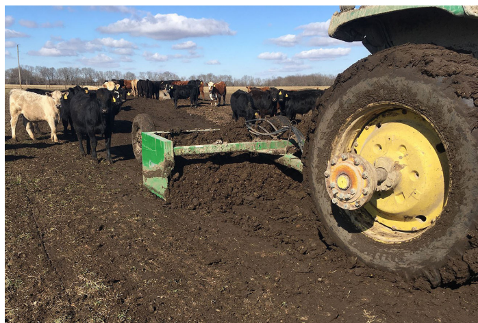
Figure 1. An example of a box scraper in use. Photo courtesy of Herschel George.
