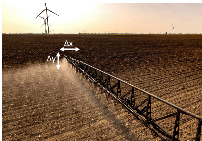
Figure 1. Types of boom motion: ( \Delta x ) Horizontal motion and ( \Delta y ) Vertical motion.
