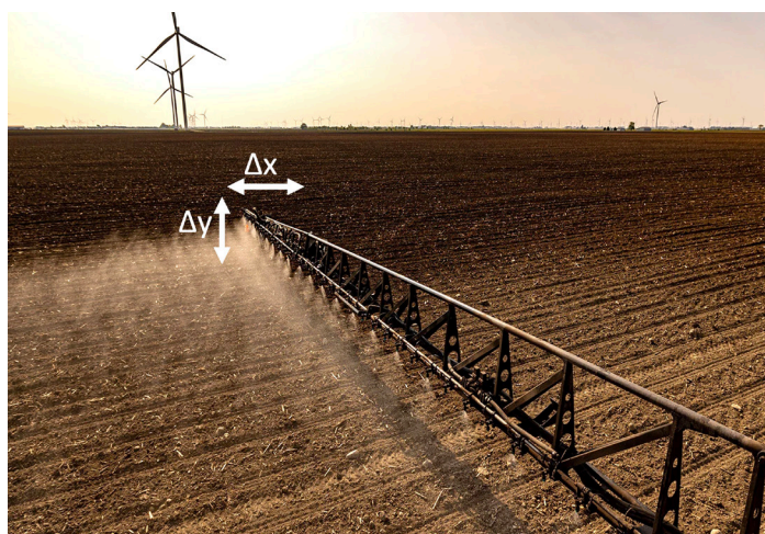
Figure 1. Types of boom motion: ( \Delta x ) Horizontal motion and ( \Delta z ) Vertical motion.
